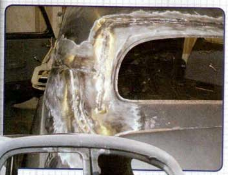
...the rear roof line was lowered by two inches. Dik says he found that relatively straight forward as the panels were easily sprung into place and welded. Note the original spot welded panel seam.
