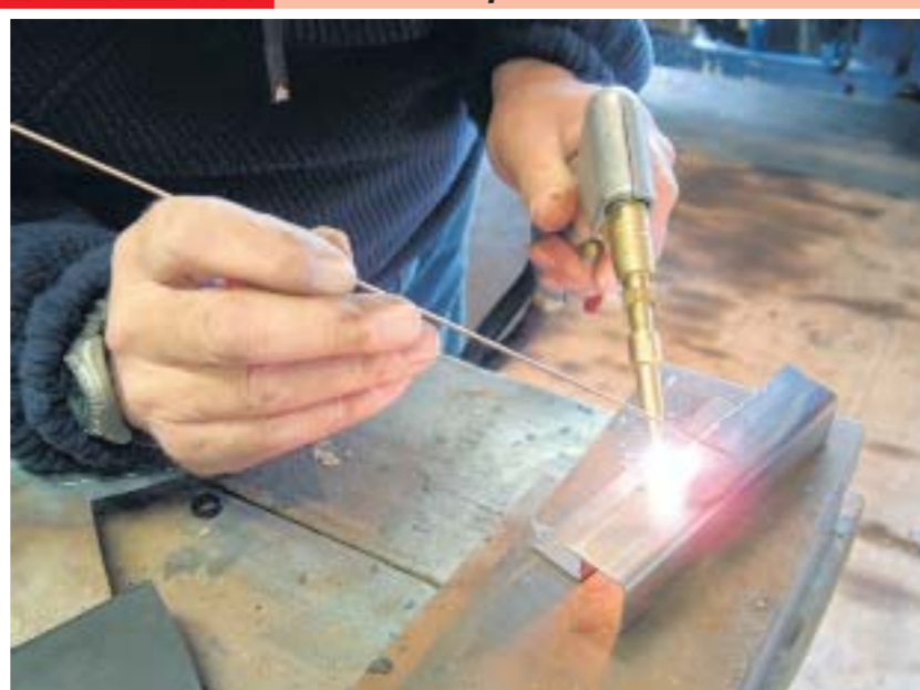
● We now have the DHC 2000 under extended test - here we see a nice delicate weld and below, our man sets up.
